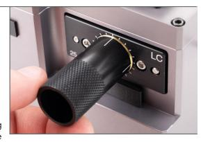
Adjusting Ring clockwise to cut closer to the ferrule face, counterclockwise to cut further away. Each calibration mark on the Adjusting Ring represents a 25 µm distance. The cut distance can be set between calibration marks for an even finer adjustment.
