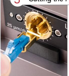
Hold the epoxied ferrule or connector at its base and carefully insert it into the Adapter Hole as far as it will go.
