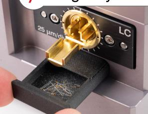
For non-vacuum models, periodically check the Waste Bin, and when necessary, safely dispose of its contents.
