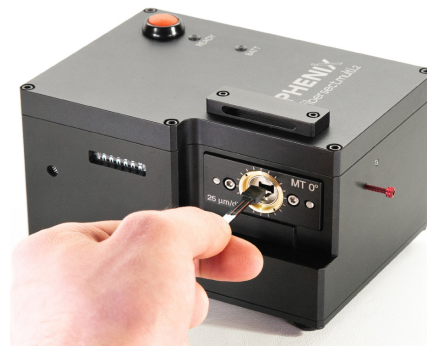
Inserting the MT ferrule
