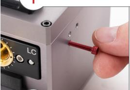
Re-install shipping screw if shipping or transporting the fibersect. Hand-tighten only.
