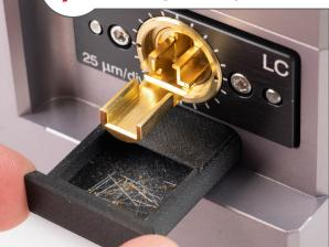
For non-vacuum models, periodically check the Waste Bin, and when necessary, safely dispose of its contents.
