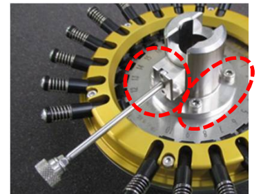
Quick Install & Release Plunger Pin (Pat. Pending) and Replaceable hub
