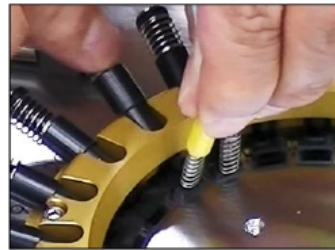
To install just simply lock down the lever after inserting MT ferrule
